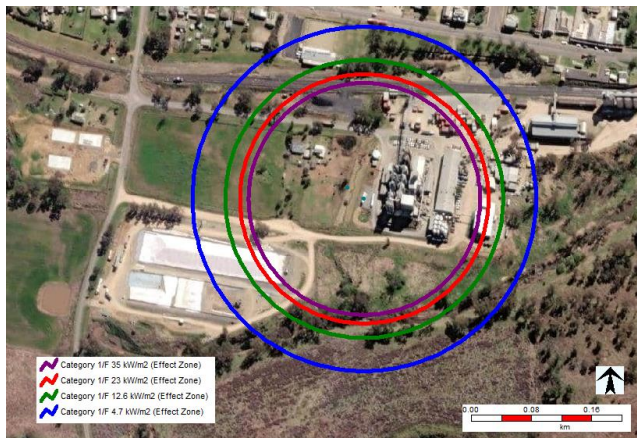
Figure 7.8 Large leak of LPG (butane) storage tank (75mm) – radiation ellipse for jet fire (Weather category 1/F)
