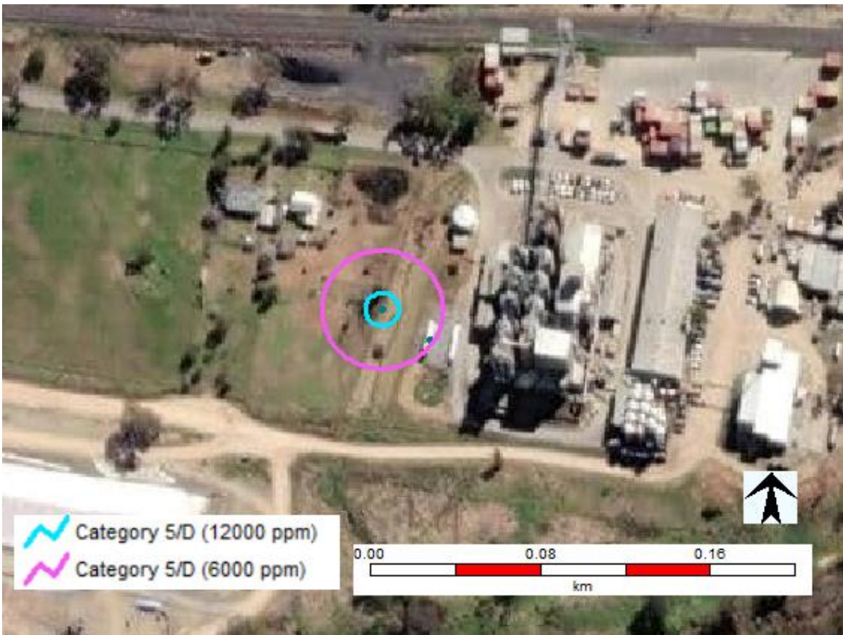
Figure 7.10 Catastrophic failure of Hexane storage tank – flash fire envelope (Weather category 5/D)
